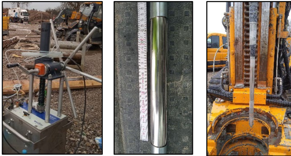
Figure 6. Control unit and mono-cellular probe of the Pencil-PMT.
