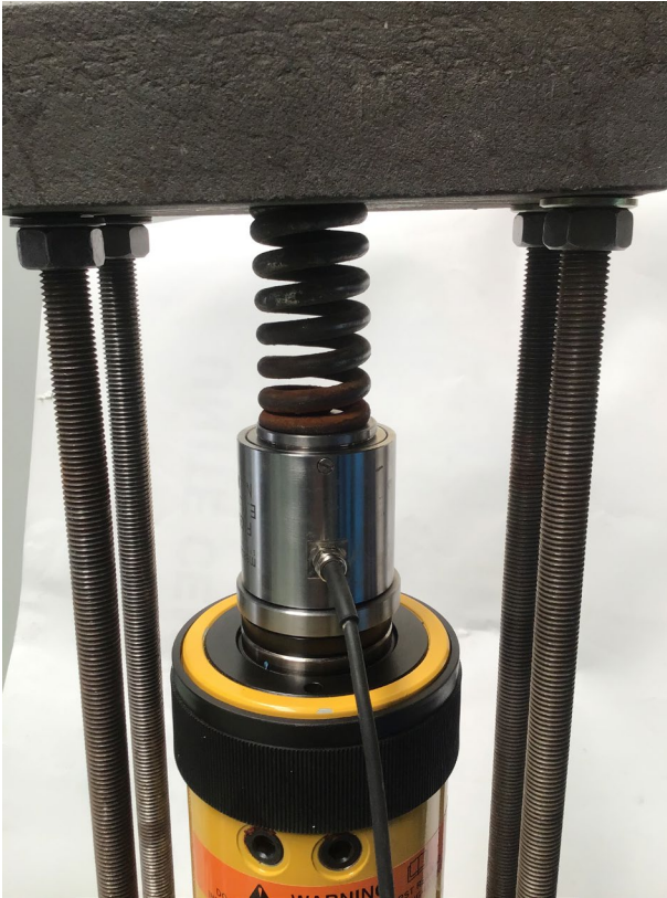
Figure 10. Spring simulation of the rise speed regulation of the cylinder actuated by a Hyperpac (result Fig.8)
