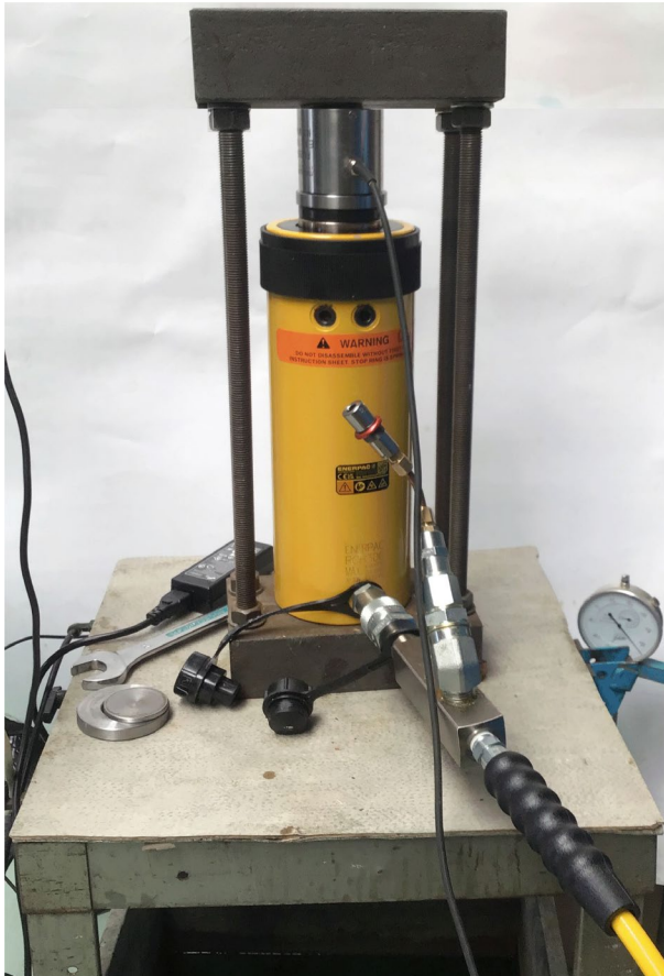
Figure 11. Pressurization of the cylinder blocked in a slightly deformable frame (result Fig.9)
