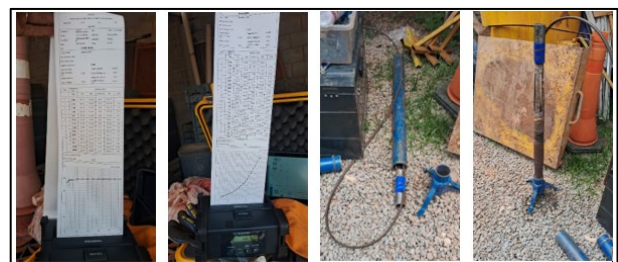
Figure 1. Pressure probe calibration process. Source: REDE Engenharia.
