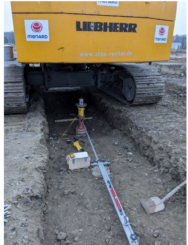
Figure 8. Single Load Test on CMC from Top of the LTP.
