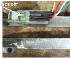
Figure 5. a) Assembly carried out for calibration, b) Ratiometric Hall Effect sensor.
