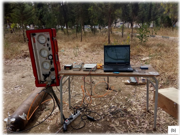
Figure 10. (a) Schematic sketch of the pressuremeter equipment on site assembly; (b) Assembly and overview on site.
