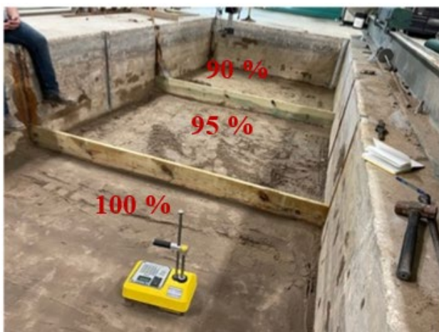
Fig. 2 FDOT-SMO indoor pit during and after fill placement (modified Proctor was adopted)
