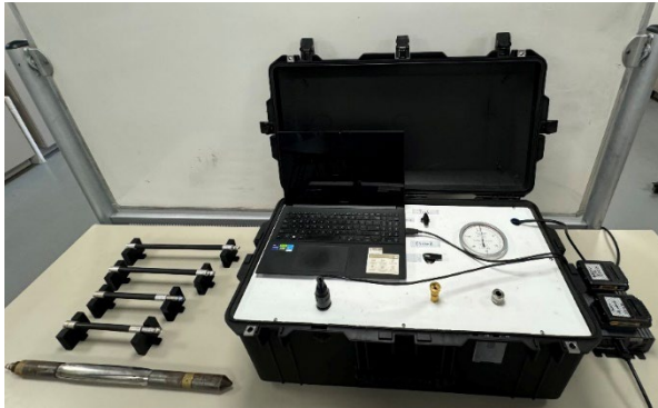
Fig. 8 The prototype of a fully automated SSMini PMT control unit
