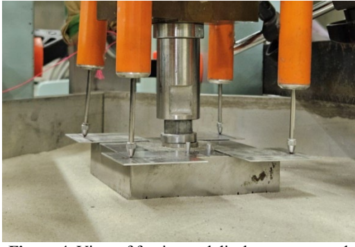
Figure 4. View of footing and displacement transducers, 2023 and 2024 equipment, in Japan
