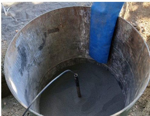
Figure 2. Calibration chamber with the pressuremeter installation prior to soil sample preparation– perfect installation.
