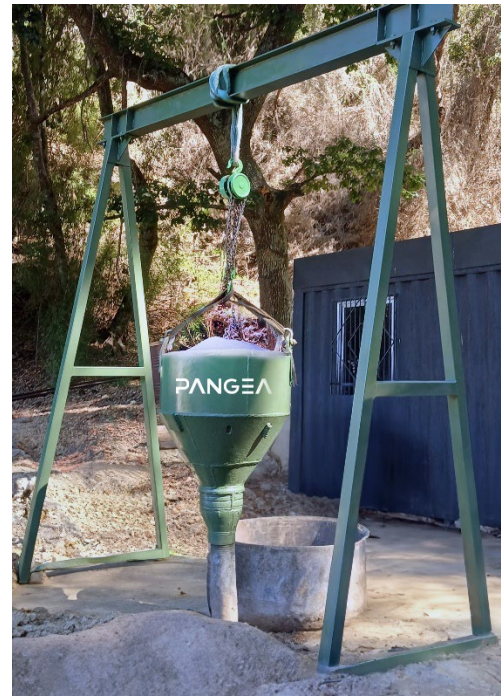
Figure 3. Container hanging from bridge crane, hose with valve.
