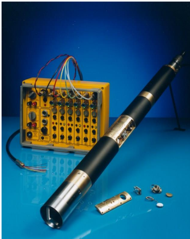
Figure 5. Six axis self boring LCPM and controller
