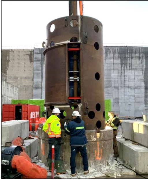
Figure 6. Site C lateral Osterberg load frame
